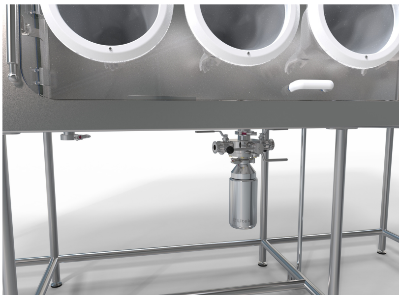
FIGURE 6. Outfeed product through split butterfly valve
